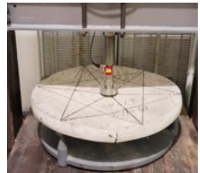
Figure 6. ASTM C1550 Shotcrete round panel test
