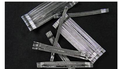
**Figure 4. Collated steel fibers**
